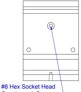
Countersunk Screw Both Sides \_\_\_\_\_
